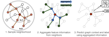
Fig. 1: Visual illustration of the GraphSAGE sample and aggregate approach [19].
