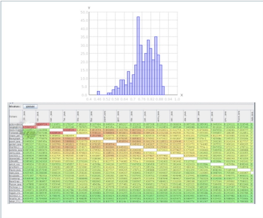
Fig. 10 Screenshots of two graphic results rendered by Baldr. On the top, the distribution of the distances measured between the codes. On the bottom, extract from the 2D visualization of the distances between each program pair (symmetrical table). The color graduation makes it possible to focus easily on the most suspicious codes
