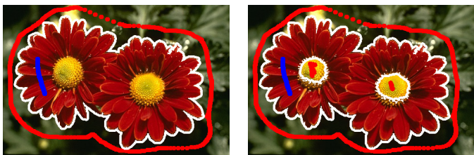
Fig. 4. Object picking with and without holes. Because we are working in the shape space, tagging the outer object is enough to recover the whole region, but it does not prevent the user to get objects with holes if he wants to.
