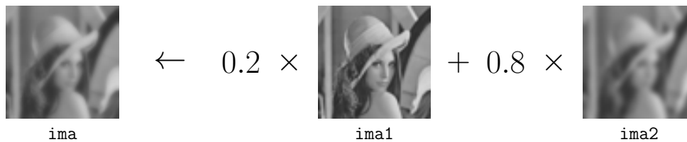
Figure 4: Alpha-blending algorithm written at image level.
