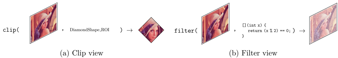
Figure 4.8: Clip and filter image adaptors that restrict the image domain by a non-regular ROI and by a predicate that selects only even pixels.
