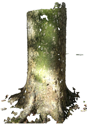
(b) 3D result using DoG, 13 images are calibrated.
