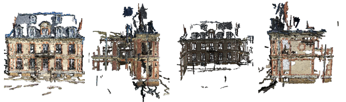
(b) Incomplete reconstructed 3D facades using DoG.
